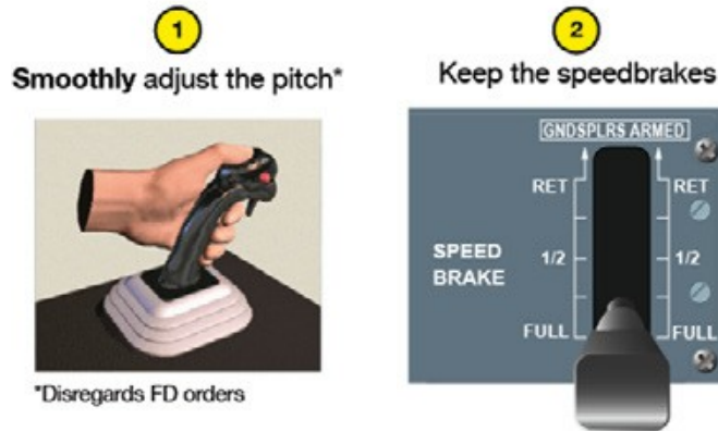
(fig.3) Actions to be taken after an AP disconnection due to HSP activation
