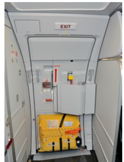
(fig.7) Removal of the decorative cover of a slide for a deployment test does not provide a realistic operational configuration.
