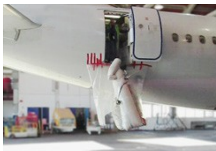
(fig.6) Incomplete inflation due to obstructed aspirator inlet caused by non-standard fuselage protection during a slide deployment test.
