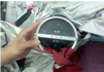
(fig.5) Aspirator flapper valve blocked in the open position due to a foreign object ingestion.
