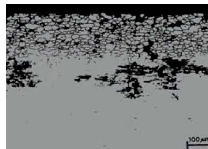
Figure 6 Example of intergranular corrosion
