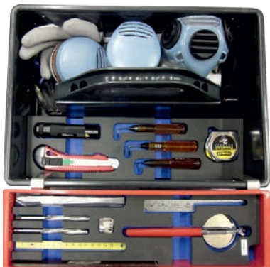
Figure 7 Tool box with shadow boards to easily detect missing tools
