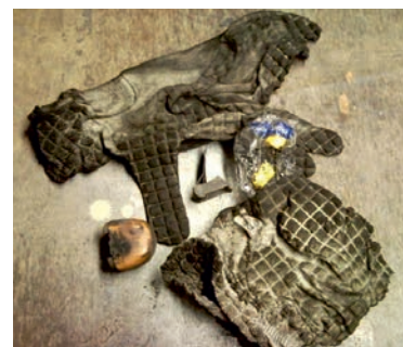
Figure 2 Foreign objects found in an APU compartment
