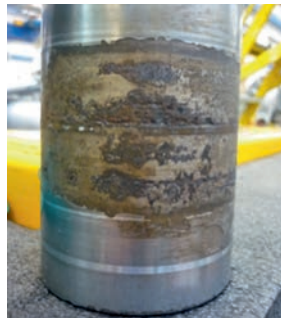
Figure 15 Water ingress to a landing gear pin led to pitting corrosion, which attacked the chrome plating and blocked the lubrication, could lead to the seizure of the landing gear
