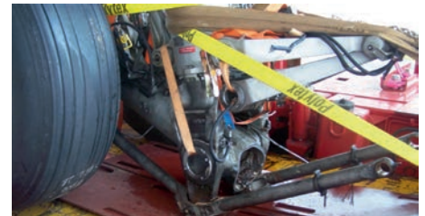
Figure 16 Pitting corrosion caused the failure of a landing gear bogie beam
