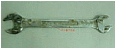
Figure 4 Wrench left in A320 horizontal stabilizer
