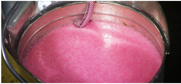
(fig.3) Foam noticed while compressing the shock absorber. Hydraulic fluid needs to be added again.
