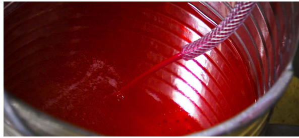
(fig.4) No foam noticed while compressing the shock absorber.
