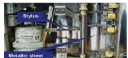
Figure 1 First generation, metal foil recorder
