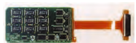
Figure 3 Third generation, solid state recorder
