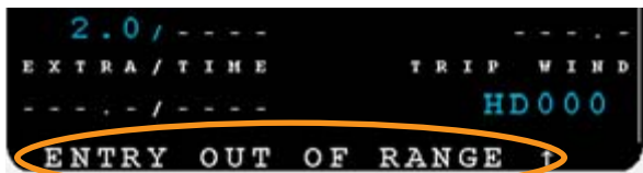
Figure 2: MCDU scratchpad message for ZFW range check
