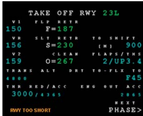
Figure 6: MCDU scratchpad message for runway limitation check (MCDU)
