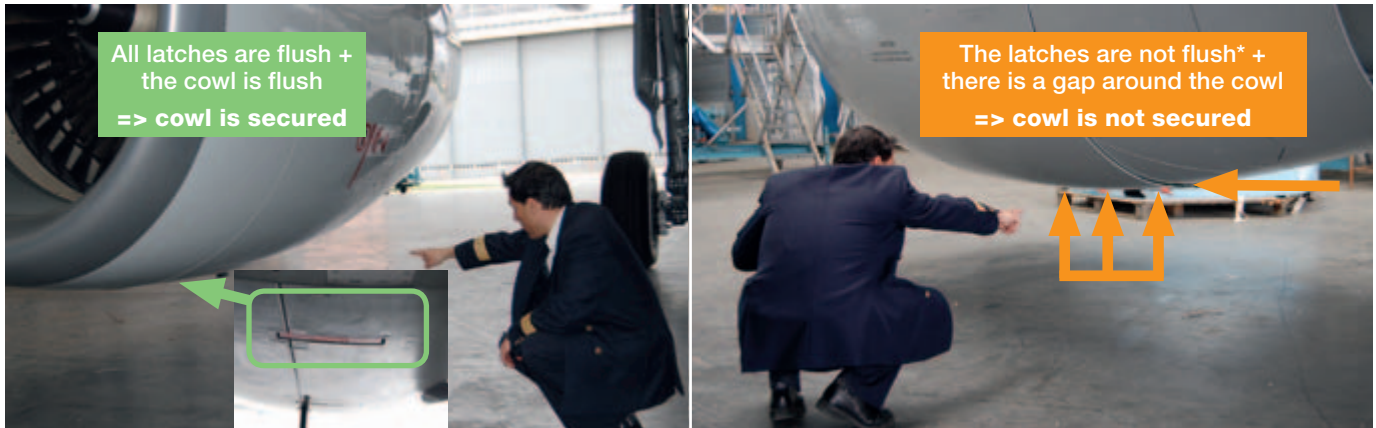
Figure 5 Proper walk-around check for secured fan cowl doors
