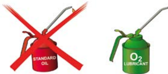
Figure 8 Use only oxygen systems approved lubricant
