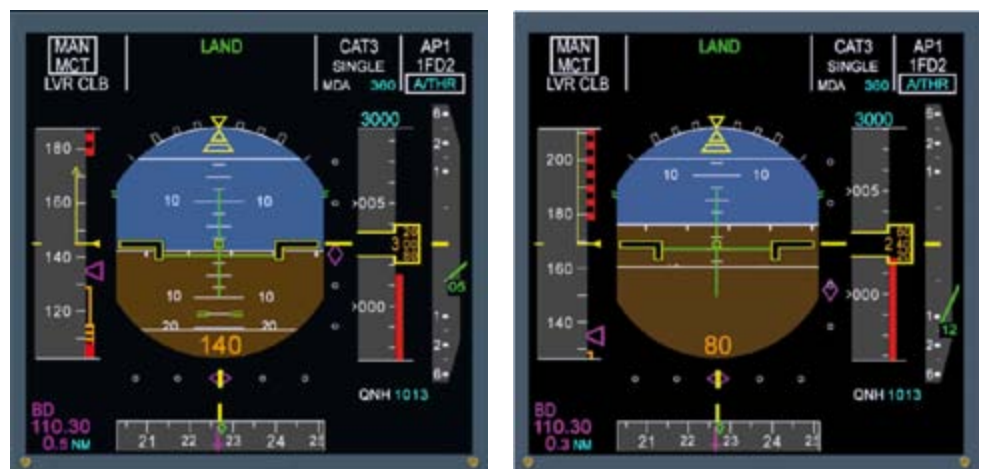
Figure 1 PFD (at 140ft and 80ft) after setting MCT instead of TOGA at 200ft during an ILS approach, (symbolic graphic – no direct reproduction of the described events)
