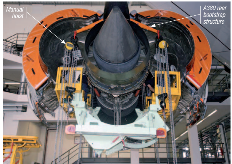
Figure 3 A380 bootstrap structure
