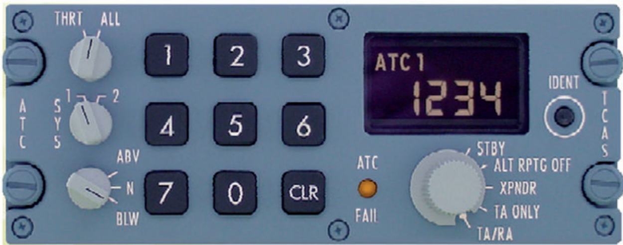
Fig 2: Gables 40 ATC/TCAS control panel
