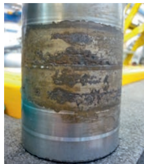
Figure 15 Water ingress to a landing gear pin led to pitting corrosion, which attacked the chrome plating and blocked the lubrication, could lead to the seizure of the landing gear
