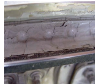
Figure 12 Corrosion between the interlaying surfaces of aerial connections could lead to loss of communication
