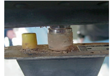
Figure 12 Corrosion between the interlaying surfaces of aerial connections could lead to loss of communication
