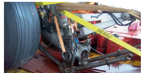
Figure 16 Pitting corrosion caused the failure of a landing gear bogie beam
