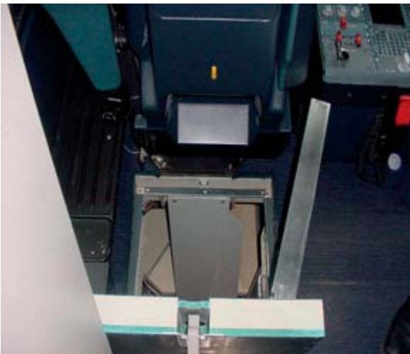
Figure 1: Open access hatch seen from cockpit door (prototype of protective arm shown)
