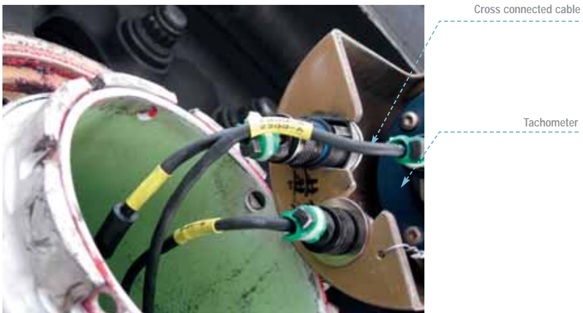
Figure 2: Picture of tachometer cross connections
