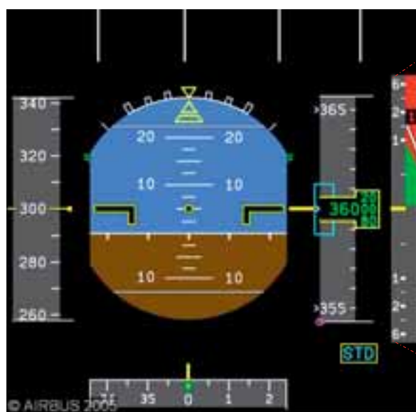
Figure 2: TCAS RA HMI without AP/FD TCAS mode
