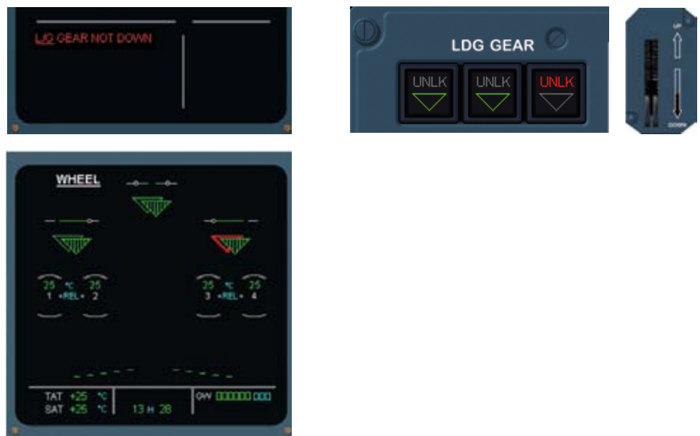
Figure 6 Illustration of spurious “ L/G GEAR NOT DOWN” indication
