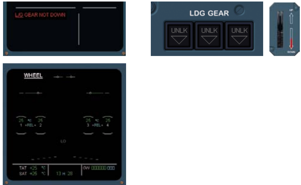
Figure 5 Illustration of “ L/G GEAR NOT DOWN” ECAM warning display – landing gear lever not selected but aircraft in landing configuration passing 750ft RA
