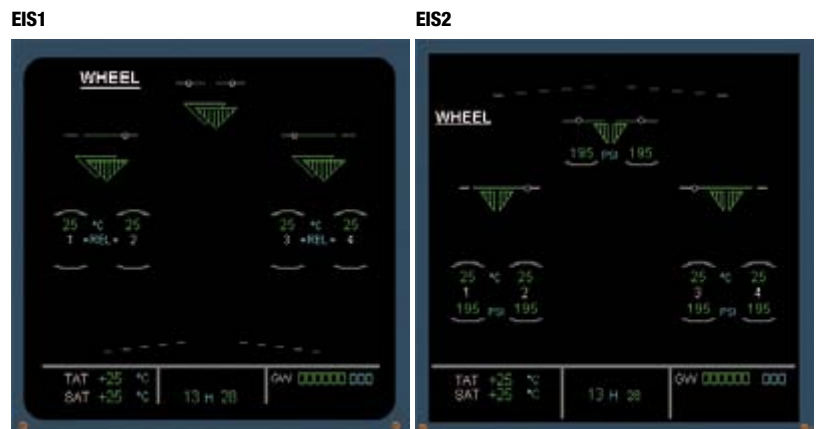
Figure 2 EIS 1 versus EIS 2 WHEEL Systems Display Page
