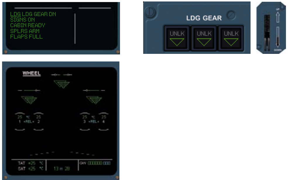
Figure 3 Normal landing gear panel and WHEEL Systems Display landing gear downlocked indications following gear down selection
